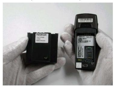
2 Put the Battery connector side into its place, and then press the Test probe side and the phone together.
